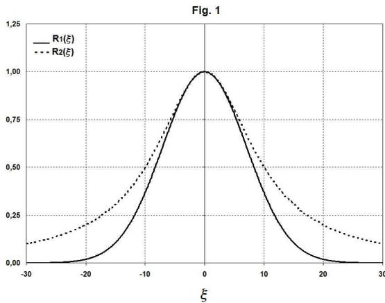
**Fig.1** - Plot of the amplitude distributions  $R_{1,2}$  assigned to the beam on the launching plane  $\zeta = 0$ , for  $\varepsilon = \frac{\lambda_0}{w_0} = 0.1$ ,
