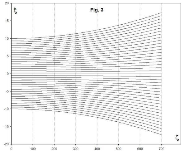
**Fig.3** - Trajectory pattern on the  $(\xi, \zeta)$ -plane, in the Gaussian case of FIG.1. The beam is truncated at  $\zeta = 700$ , in order to limit it to its most interesting part.
